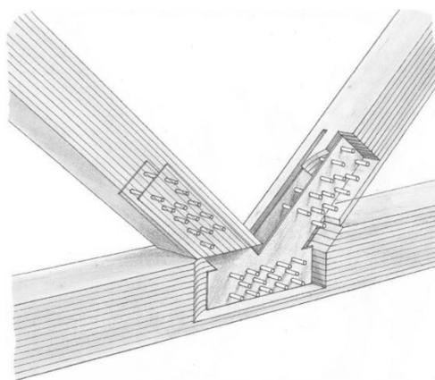
All glulam elements are connected by use of slotted-in steel plates and dowels, see figure to the left. This is a high capacity connection, which is commonly used in bridges and
