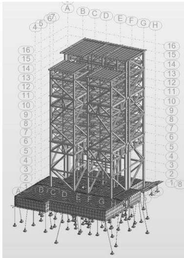
[4] gives guidelines on how to calculate the peak accelerations. [5] gives recommended design criteria for wind-induced vibrations to evaluate the serviceability of the building. [6] also gives guidance for human response to vibrations. To analyze the dynamic behaviour of the building a FEM-model was made using Robot Structural Analysis Professional 2013. The global model is shown to the left.
