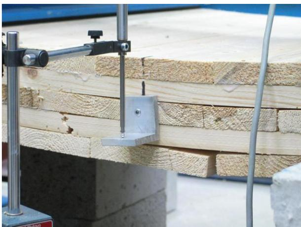
**Figure 7:** Flexure collapse mode for BTOD-3 specimen.
