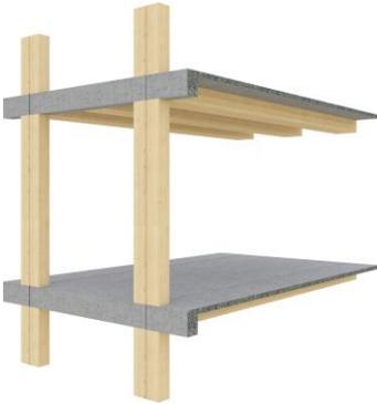
*Fig.5: Loadbearing system*
